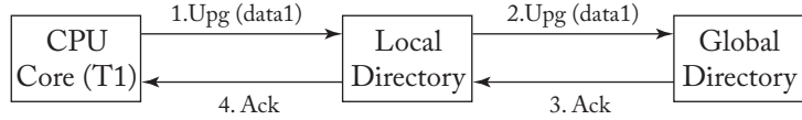
Figure 10.6: Stitching together a consistency-agnostic protocol with a consistency-directed one: Coherence transactions for St1 from the CPU.
